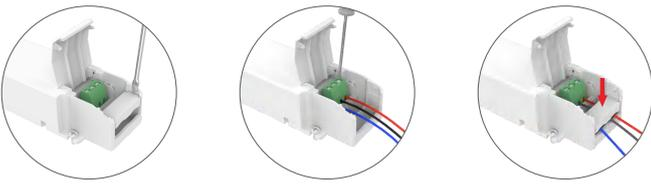
Use a screwdriver to pry up the protective housing at the edge of the wire fixing board. Then connect to the wires as the diagram shows and press down the wire fixing board.
