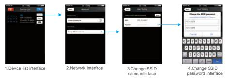
[Attn]: In direct connection of the WiFi-103 as a router. Please exit software after changed the SSID name and the password, then enter the mobile device system setting to reconnect the WiFi-103, In additional wireless router connection, it only needs to click " " in Device List interface to search again the WiFi-103 controller after changed SSID name.
