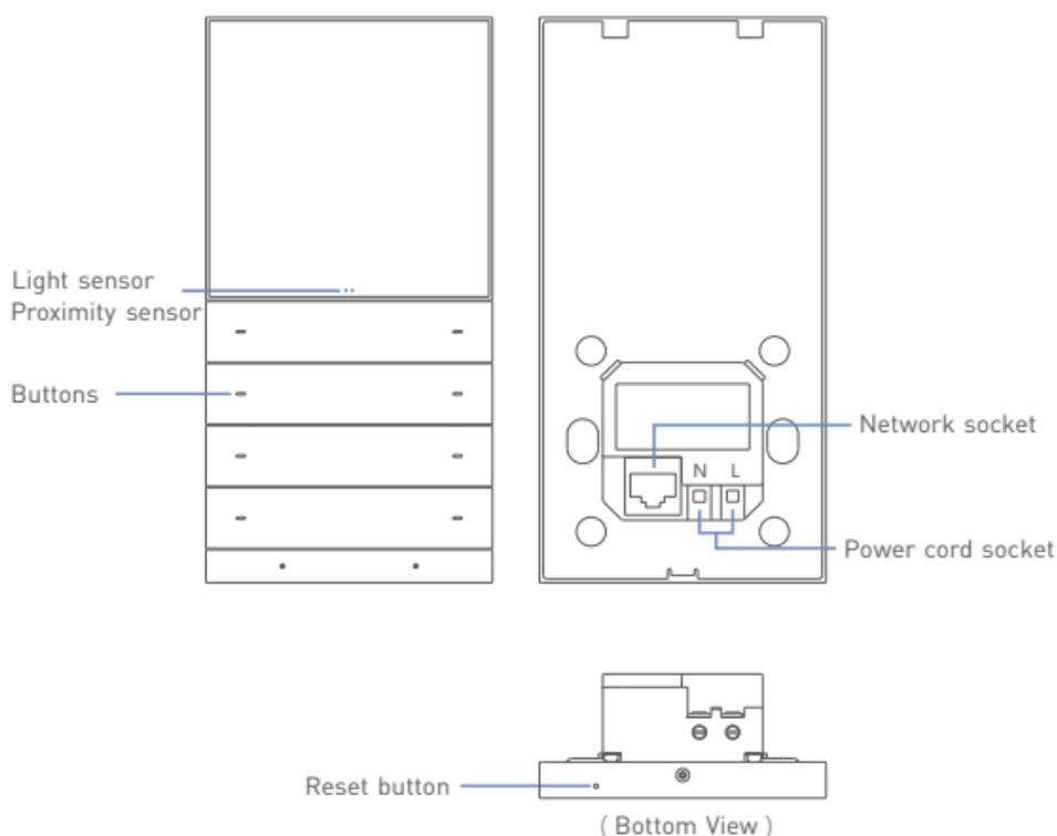
\* Reset button: Long press it for 16s until the screen turns on and displays the LTECH LOGO.
