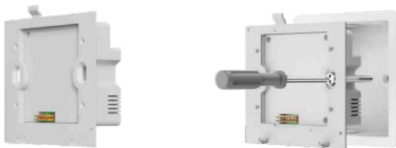
4. Slant the bottom of the panel cover and snap it to the panel frame. Then secure the panel cover to the frame from the bottom with a KM2 screw.
