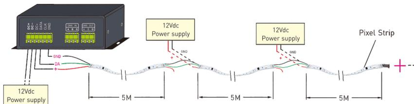
B. Special connection method - light fixtures and controller using different operating voltages.
