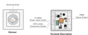
Working Temperature: Switch Dimensions: Remote Dimensions: Packaging Dimensions: Weight (G.W): -30°C~55°C L87×W87(mm) L86×W33(mm) L96×W91×H61(mm) 175g
