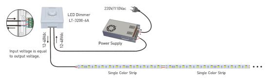
5.2 Offer PWM dimming signal to drive other equipment:
