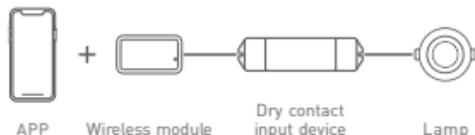
2. Both App and remote can control the wireless module after connecting the remote to wireless module via App.
