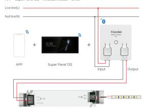
Wireless module + Multiple Phase cut power amplifiers + Multiple Phase cut LED drivers
